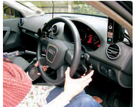
Raquel's car showing hand controls and the controls for the roof top wheelchair storage
