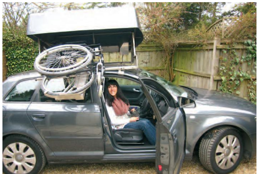
Raquel controls the hoist's descent from the top box and positions her chair for pick up. The folded wheelchair is lifted into the roof box
