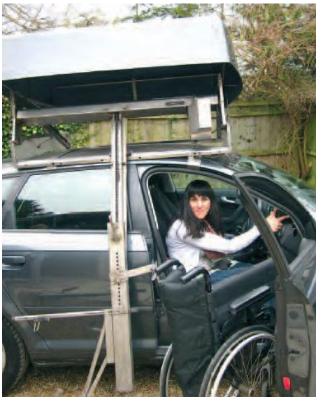
Raquel controls the hoist's descent from the top box and positions her chair for pick up. The folded wheelchair is lifted into the roof box
